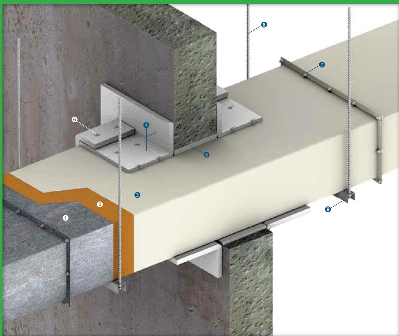
For FRL of 120 minutes Integrity only (Duct A & B) in accordance with BS476: Part 24: 1987
